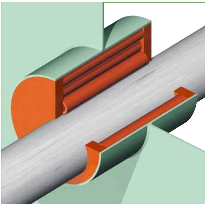
The NOFIRNO® sealing system is certified for A-0 and H-0 class without the use of any insulation. In these cases, the only difference is that the conduit depth is 250 mm instead of 180 mm. NOFIRNO® sealant with a thickness of minimum 20 mm to be applied at both sides. System is also gas and watertight.
