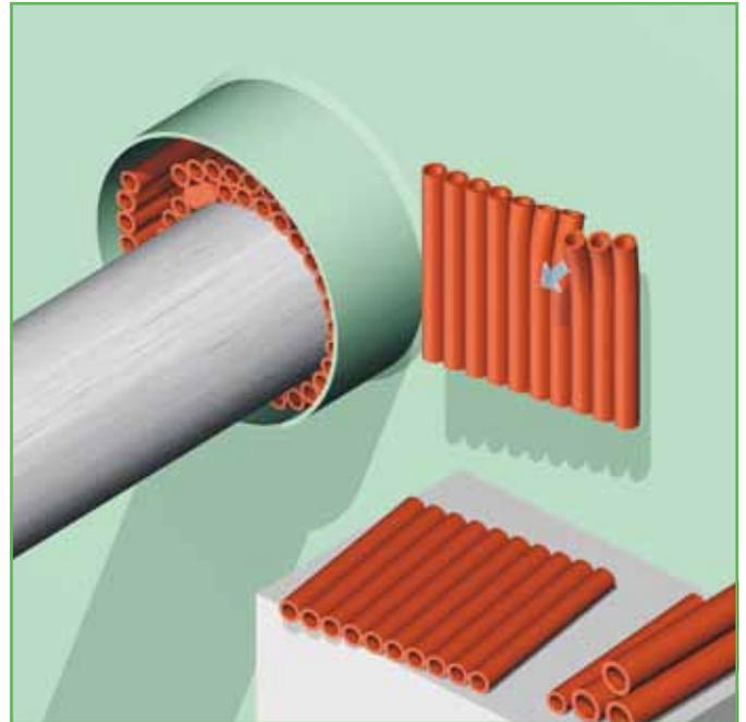
For oversized conduits and/or off centre ducted pipes, a combination of NOFIRNO® single and multi-filler sleeves can be used. NOFIRNO® sealant with a thickness of minimum 20 mm to be applied at both sides. Conduit depth minimum 180 mm.
