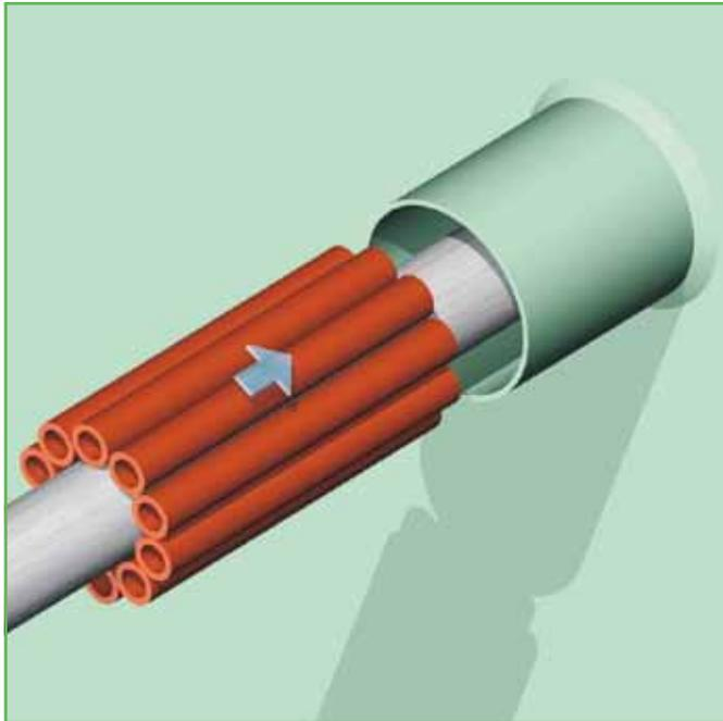
Several options are available with the NOFIRNO® sealing system. The most simple and cost effective solution is a fitting multi-filler sleeve applied in a conduit sleeve with an ID creating a tight fit. NOFIRNO® sealant with a thickness of minimum 20 mm to be applied at both sides.
