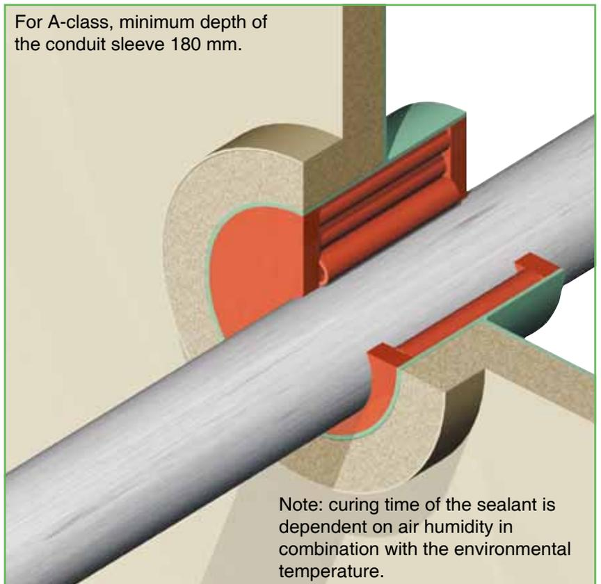
Note: curing time of the sealant is dependent on air humidity in combination with the environmental temperature.
