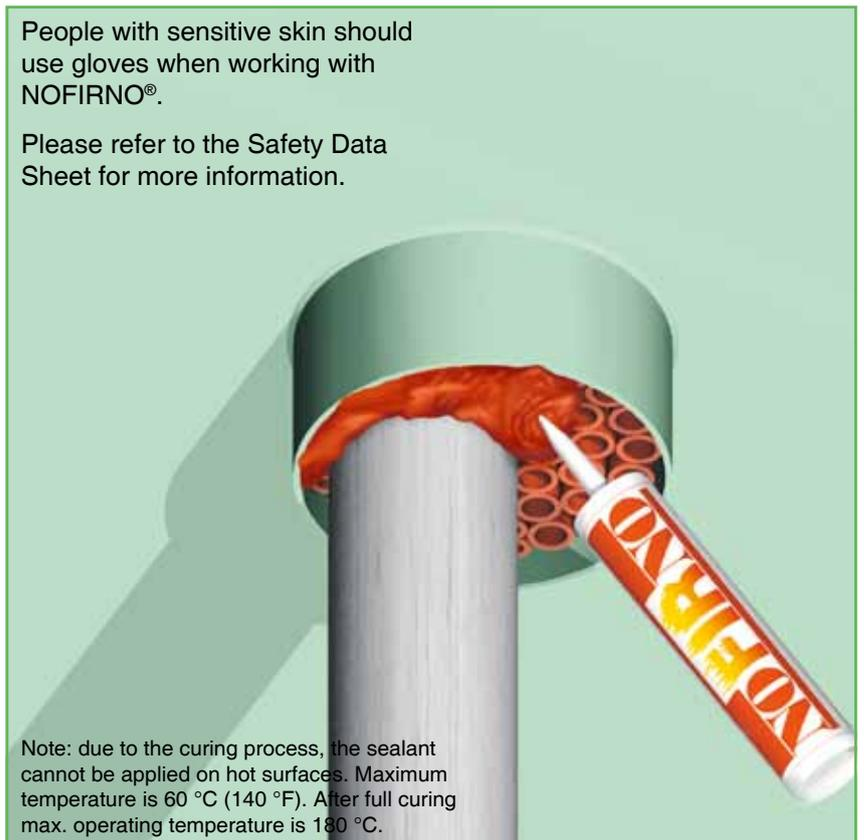
Note: due to the curing process, the sealant cannot be applied on hot surfaces. Maximum temperature is 60 °C (140 °F). After full curing max. operating temperature is 180 °C.
