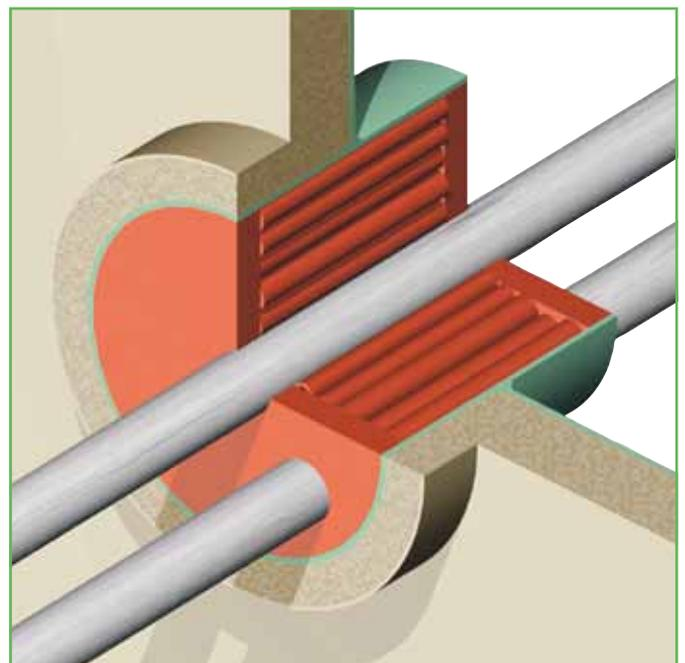
The NOFIRNO® sealing system is also approved for multi-pipe penetrations of steel, copper and GRP pipes to a transit size of 1000x300 mm with a depth of 180 mm only. Minimum separation of the pipes to be regarded. NOFIRNO® sealant with a thickness of minimum 20 mm to be applied at both sides.
